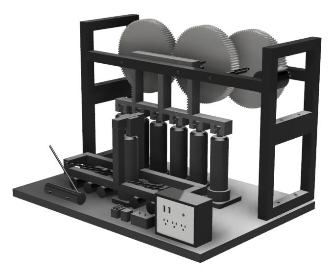
In the third system, the Bannon Maher Leveraged Generator and Motor, an axle to power a generator and or function as a motor is spun by the force generated by hydraulics. A commodity hand operable hydraulic cylinder and pump, can generate force of 100,000 pounds, with the hydraulic pump handle powered by an electric motor.
